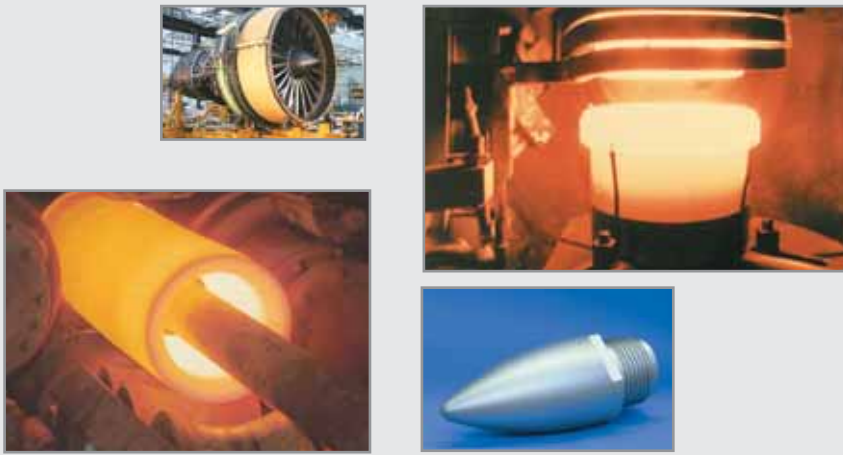
Figure 7. Traditional molybdenum applications in hot metal forming. Upper right: TZM and MHC isothermal forging die components used to manufacture aircraft gas turbine (upper left) components. Lower right: TZM piercing plugs for the manufacture of pierced stainless steel tubing (lower left). Courtesy of PLANSEE Metall.
